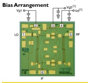
**App Note [1] Biasing** - As shown in the bonding diagram, the pHEMT mixer devices are operated using a separate gate voltage Vg1.Set Vg1=-0.6V for optimum conversion loss performance. pHEMT test device (Vd,Vg2) with 100 Ohm resistor is provided so that mixer gate bias can be corrected for local Vto.
